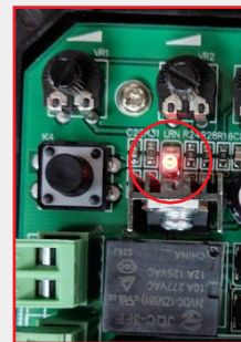
The Learn LED will flash repeatedly and then turn OFF. when the remote is paired.
