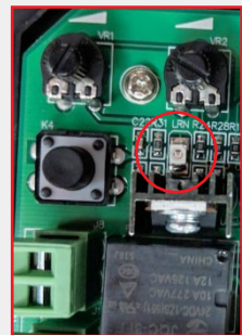
The Learn LED will flash repeatedly and then turn OFF. when the remote is paired.
